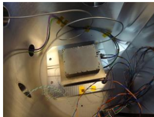
X-band transmitter TVAC testing
