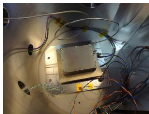
X-band transmitter TVAC testing
