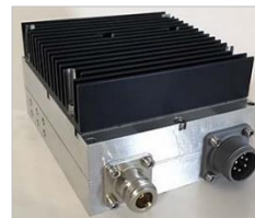
RF signal processing HW (X-band downconverter)
