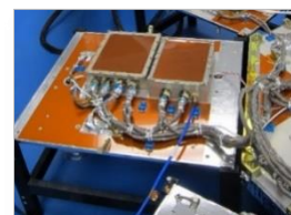
Flight heritage: 1 st gen. X-band TX payload - TRL9 in 2021 (NEMO-HD mission, @SPACE-SI 2020).
