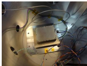
X-band transmitter TVAC testing
